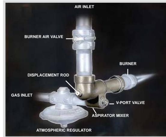
Figure 1. Typical arrangement of 3065 Aspirator Mixer with burner, atmospheric regulator, and air valve.
