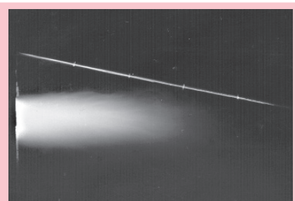
Gas (left) and light oil flames for 6514-6 Dual-Fuel Burner with 16 osi main and atomizing air pressure drop across burner. White lines on pipe above flame indicate 1' intervals.
